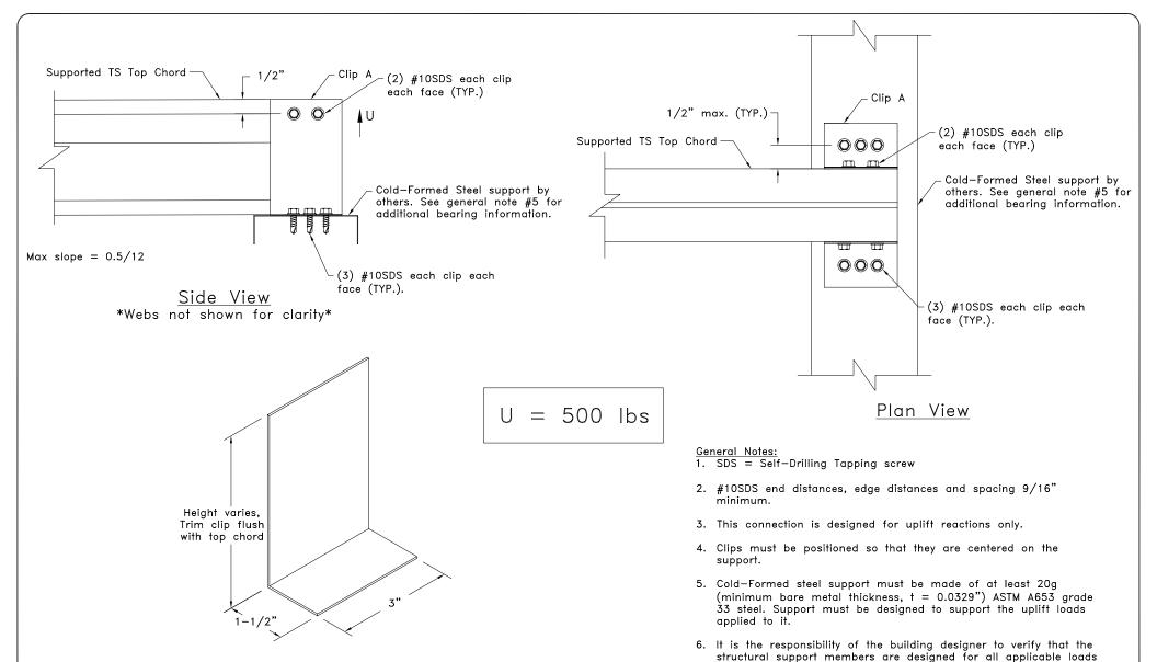
Clip A 16g ASTM A653 SS Grade 33 G60 Bare metal Thickness: t = 0.0538"
